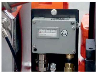
Ex Shut down pressure switch.
