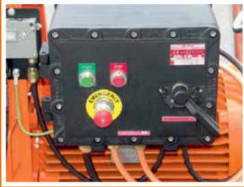
Cast electrical Eex box with main switch, star delta starter and overload relay.
