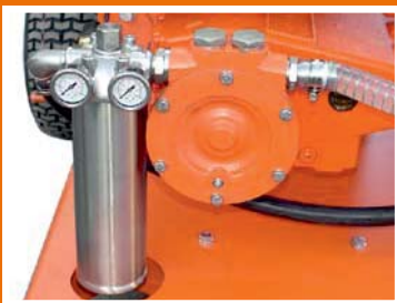
Integrated booster pump & filter system.
